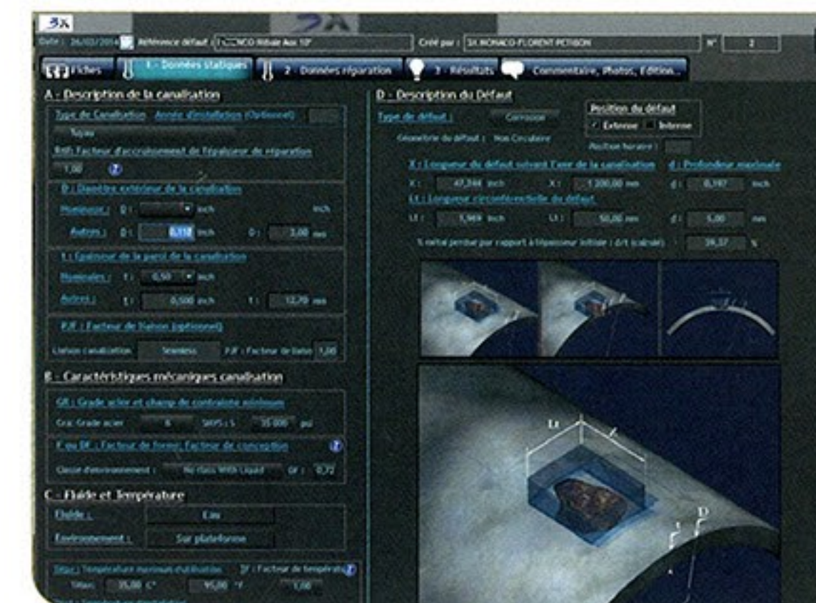
R.E.A (Reinforcekit Engineering Analysis) for repair dimensioning: length and numbers of layers according to ISO 24817 & ASME PCC2
