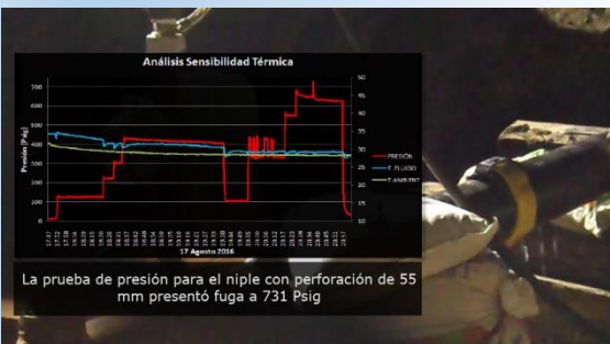
Figure 3: Pressure test for 50mm hole → leaks at 731 psi
