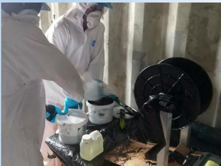
Figure 3: Kevlar tape impregnation with resin using BOBiPREG
