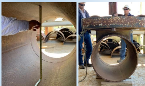
Figures 3-4: Measurement of inner diameter and initial loading
